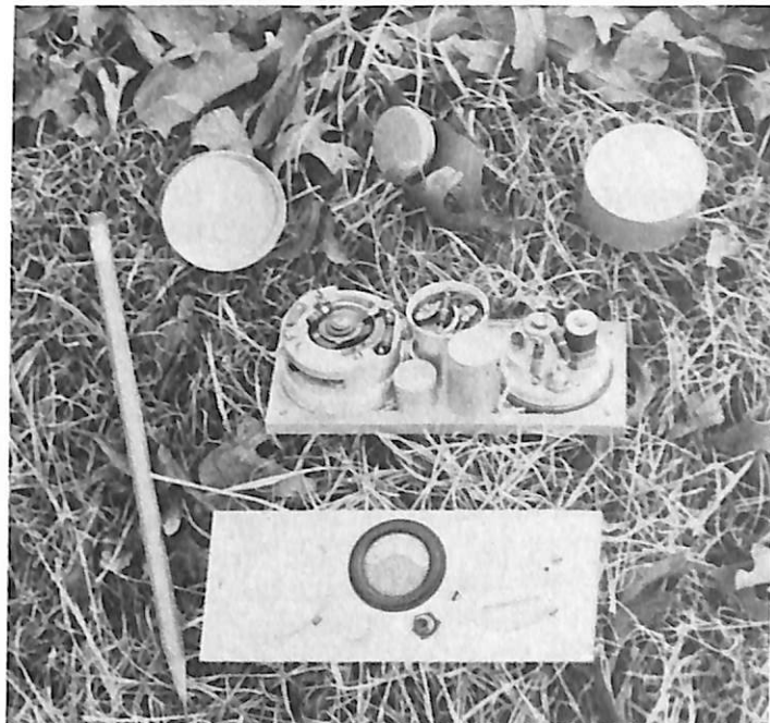
Figure 135. A signal generator designed by Wilbur Claypool and milled by him from aluminum stock at the Forest Service Electronics Center. (Forest Service photo, History Section)
