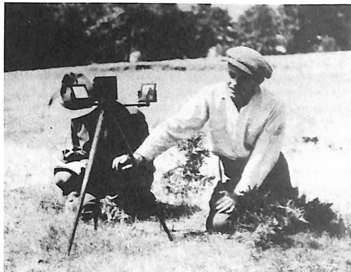
Figure 12. Sending messages to and from lookout points by heliograph. Above, single tripod type, Klamath National Forest, northern California, October 1921. Below, double tripod heliographs in use by the Forest Service on a peak in the West, ca. 1915. (NA:95G-159767, 30847A)
