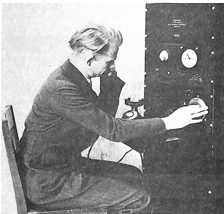
Figure 60. Logan Belleville, who designed it at the Radio Laboratory in 1936, is at the controls of a type U-30-25 fixed-base vhf radiophone with output power of 20 watts, in the Region 6 headquarters in Portland, Ore. (Forest Service photo, History Section).
