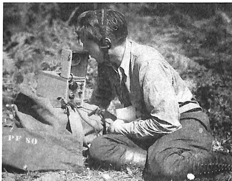
Figure 43. Demonstration of the type PF voice radio set, developed in 1933 by Squibb and Lawson at the Radio Laboratory. (NA:95G-280931)
