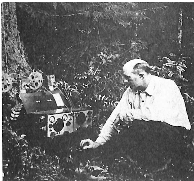
Figure 23. Dwight Beatty operating the SP-1929 set he designed -- the first successful lightweight low-power radio receiver-transmitter tested in heavy timber. (NA:95G-250701)
