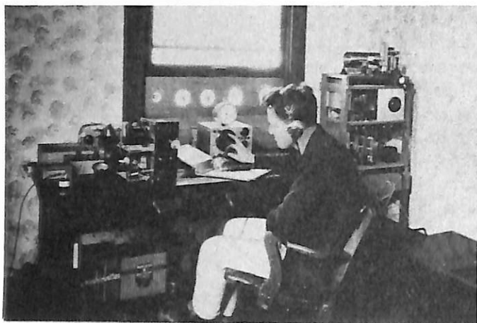
Figure 36. Harold Lawson testing a semiportable model he designed at the Radio Laboratory in Vancouver, Wash., late in 1931. In the corner is his 50-watt transmitter model; it was also used as the control station on the Columbia (now Gifford Pinchot) National Forest during the 1931 fire season. (NA:95G-262294)
