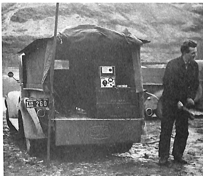
Figure 69. SPF model set up for semi-portable use at a Region 6 temporary base camp. (Forest Service photo, History Section)
