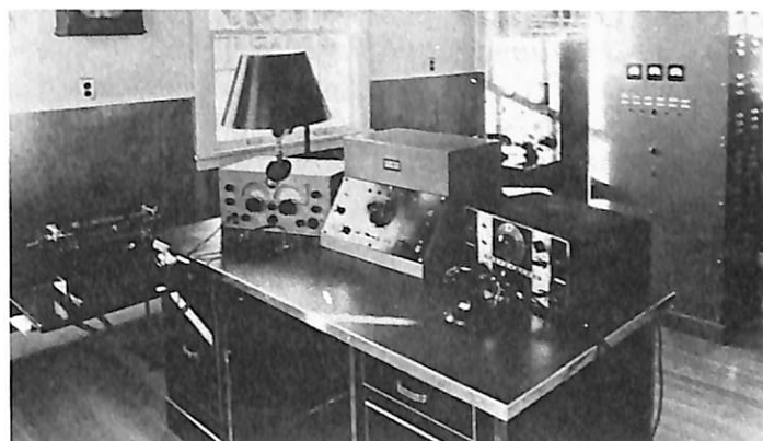
Figure 64. Transmitting and receiving equipment at the Radio Laboratory's Station KBAA, Portland, Ore. A new 250-watt transmitter installed about 1939 kept the Laboratory in close touch with personnel on field assignments. (Forest Service photo, History Section)
