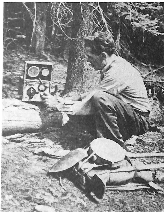
Figure 120. A fire scout with his lightweight SPF set. Note pulaski (grubhoe-axe firefighting tool), shovel, canteen, and bedroll in foreground. (Forest Service photo, History Section)
