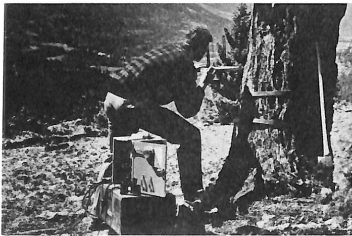
Figure 102. Field demonstration of the Radio Laboratory's SP (semiportable) radio by Richard Ogg of Region 1 mobile radio unit (Station W7AOD), at a temporary lookout station, ca. 1933. Ogg is using alidade (fire locator) attached to tree. Note binoculars on equipment kitbox, which was used to carry the SP set, antenna, and heavy-duty batteries required for semipermanent locations. (Forest Service photo, History Section)
