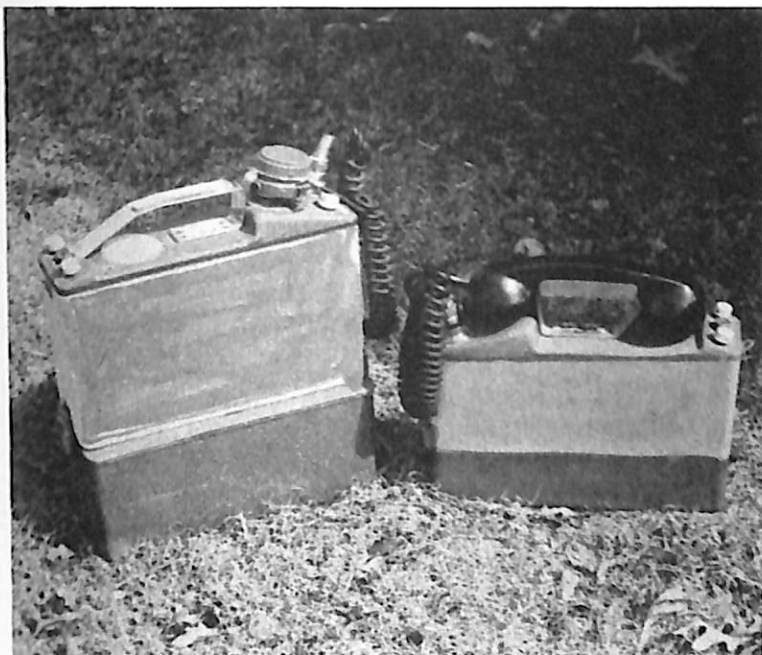
Figure 132. Handie-talkies, made by the Motorola Corporation, were purchased by the Forest Service under competitive bid in the early 1950's after precise specifications for the sets were completed by the Radio Laboratory. At left, model P31BAC-1061AM. At right, model H-21-3. (Forest Service photo, History Section)
