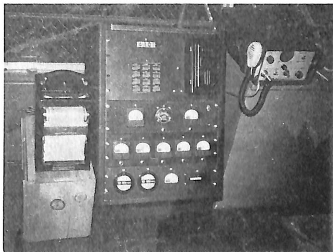
Figure 138. Instruments of the remote Forest Service radio relay repeater station powered by solar energy cells at a test installation in California. Developed by Guy Wood, shown left to right are strip chart recorder, special instrumentation, and the Motorola repeater unit. (Forest Service photo, History Section)
