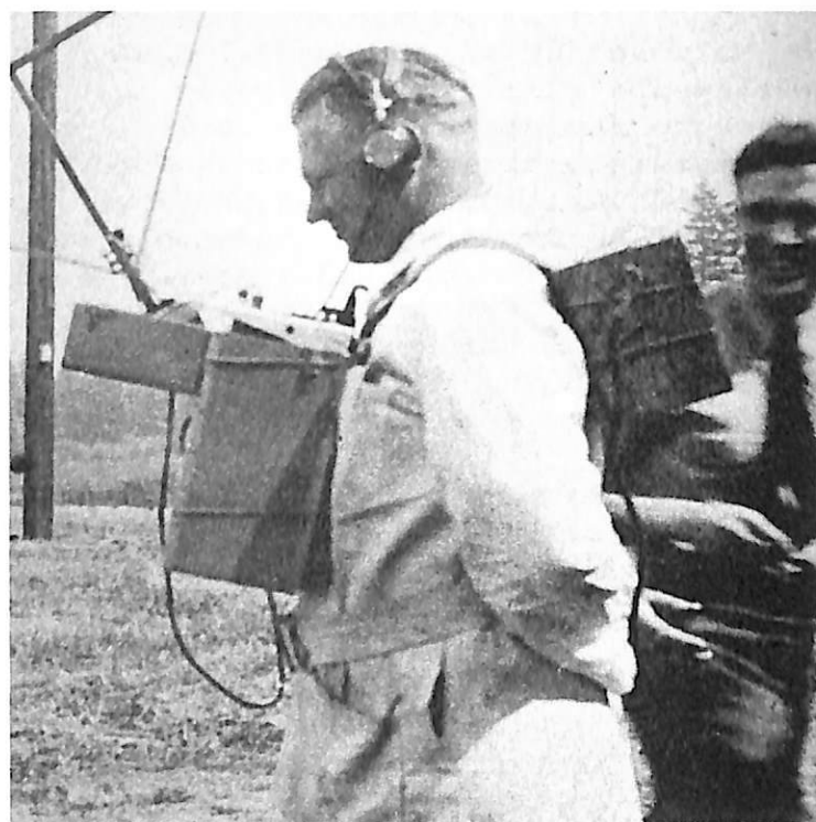
Figure 82. Ralph Kunselman demonstrates the experimental type X metal detector developed by the Radio Laboratory, while Harold Lawson looks on. The gadget was designed to warn sawyers of nails, bolts, spikes, wire, etc., in logs they were processing after the New England hurricane of 1938. The work came under the timber salvage program of the Forest Service and cooperating States. (Forest Service photo, History Section)
