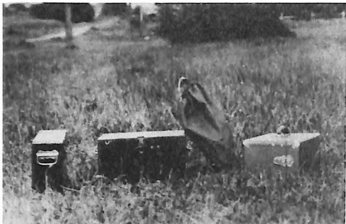
Figure 27. The SP-1930 packed for travel. At left, equipment case, 11 pounds, 11 ounces. Center, battery case, 44 pounds, and sack of antenna equipment, 5 pounds, 12 ounces. At right, transmitter-receiver, 17 pounds, 14 ounces. (NA:95G-249318)
