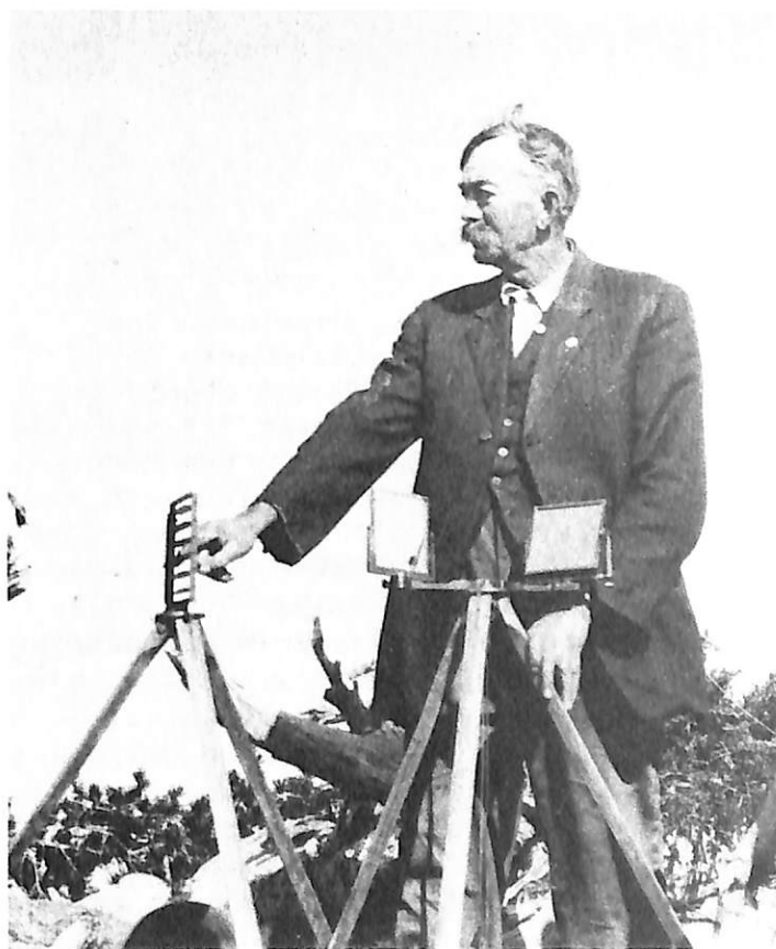
Figure 12. Sending messages to and from lookout points by heliograph. Above, single tripod type, Klamath National Forest, northern California, October 1921. Below, double tripod heliographs in use by the Forest Service on a peak in the West, ca. 1915. (NA:95G-159767, 30847A)
