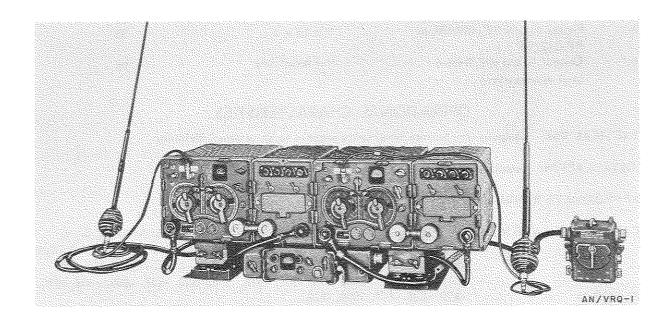
Radio Set AN/VRQ-1 is a short-range, vehicular, f-m (voice) equipment for point-to-point, retransmission, or radio relay communication within and between armored units or between armored and artillery units.
