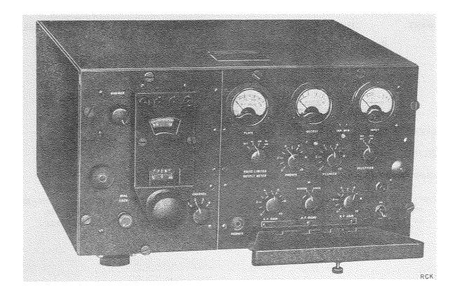
Radio Receiving Equipments RCK and RCK-a are a-m (voice, mcw) v-h-f receivers used in conjunction with VHF Radio Transmitting Equipment TDQ on aircraft carriers and at shore stations for communicating with aircraft.
