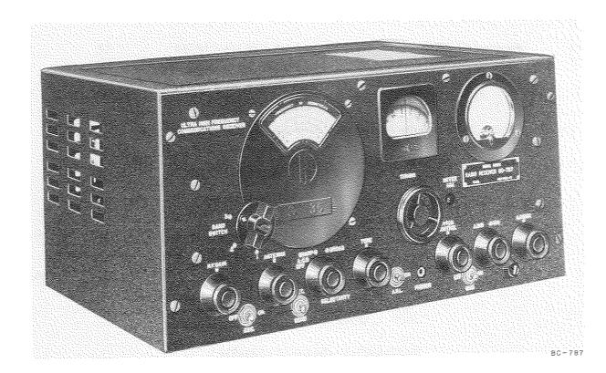
Radio Receiver BC-787 is a 3-band, a-m and f-m, voice and c-w equipment operating in the v-h-f range. It can be used in fixed plant point-to-point communication, for intercept or monitoring purposes, and for special applications in vehicles as a mobile equipment.
