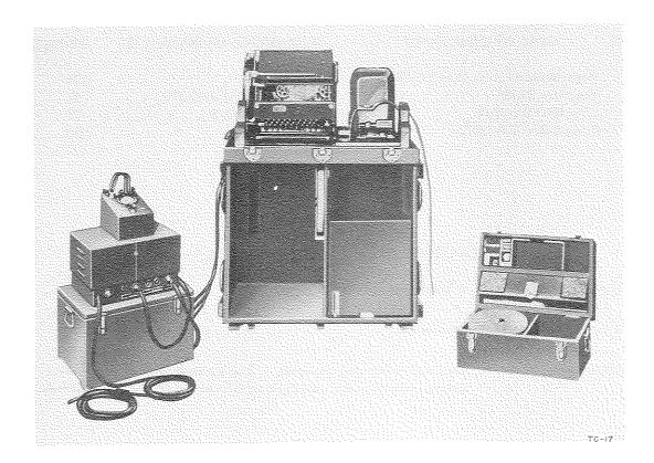
Reperforator-Teletypewriter Set TC-17 (the weather communication version of Reperforator-Teletype-writer Set TC-16) is a transportable, field, automatic tape sending and receiving teletypewriter station equipment used for transmission and reception of weather data at air station of division and higher headquarters.
