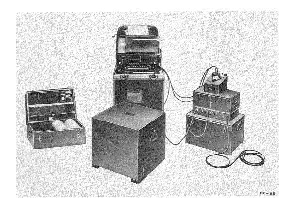
Teletypewriter Set EE-98 is a complete, transportable field teletypewriter station which requires only connection to power and communication lines in order to operate. It is used by battalian and higher headquarters.
