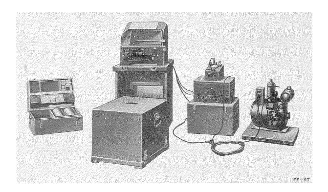
Telegraph Printer Set EE-97 is a complete transportable, field teletypewriter station used for transmitting and receiving telegraph communications at battalion and higher headquarters.
