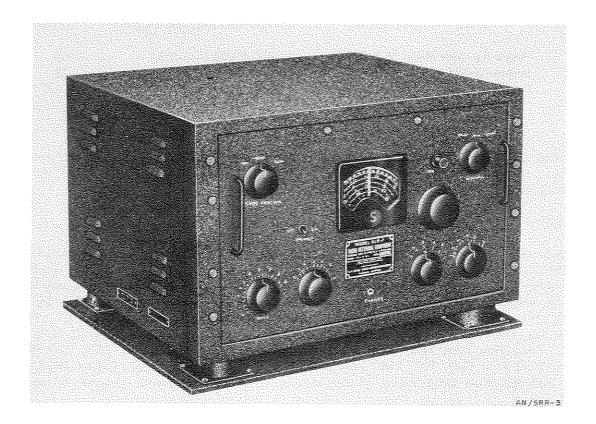
Radio Receiving Set AN/SRR-3 is a medium-range, a-m (voice, cw, and mcw) receiving equipment for radiotelephone and radiotelegraph communication in the I-f, m-f, and h-f ranges and is used on shipboard and at fixed shore stations.
