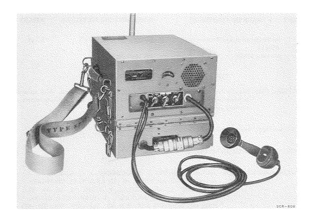
Radio Set SCR-609 is a transportable, low-power, short-range, f-m (voice), transmitting and receiving equipment used by field artillery units.
