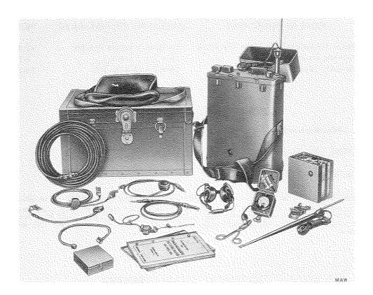
Portable VHF Radio Transmitting and Receiving Equipment MAW is a low-power, v-h-f, pack type communication set used in ground-to-air liaison, ship, or shore based emergency communication. The entire equipment, including accessories, is contained in a portable submersion-proof case. It is capable of voice and mcw transmission and reception on any one of 10 preset crystal-controlled channels.
