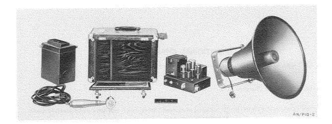
Public Address Set AN/PIQ-2 is a portable, medium-power, general purpose sound amplifying and projecting equipment used for beach control purposes during amphibious operations, for control of groups of personnel, and similar tactical applications.
