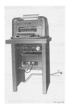
Teletypewriter TT-61/FG is a transportable, page-printing, standard communication, sending and receiving teletypewriter station equipment used at permanent or semipermanent camps, posts, and stations.
