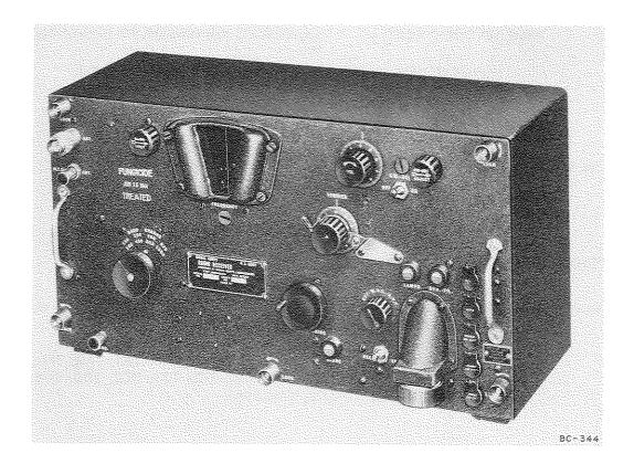
Radio Receiver BC-344 is a lightweight, portable, a-c operated, a-m radio receiving equipment used for voice, c-w, and tone signal communication in the low-and medium-frequency bands. It is a general purpose equipment which is widely used in fixed plant applications at higher headquarters and for special purposes.
