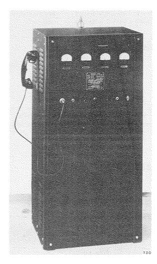
Radio Telephone Transmitting Equipments TDD and TDD-1 through -4 are single-frequency, low-power, a-m (voice) transmitters for use in airport traffic control towers.
