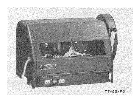
Reperforator TT-53/FG is an automatic tape-perforating and typing teletypewriter receiving equipment used for production of message tapes which may be distributed later by a transmitter-distributor to line circuits or to local page printers. It prints English characters.
