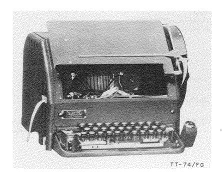
Teletypewriter Reperforator TT-74/FG is sending and receiving teletypewriter station equipment which produces typed and perforated paper tape of messages received from the line and which can transmit to the line from tape so produced. It can be used in tape-relay and torn-tape switching applications and for monitoring where a permanent record of messages is needed.
