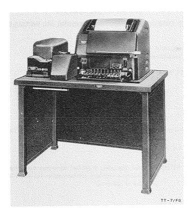
Teletypewriter TT-7/FG is a standard communication, page-printing, tape-perforating and transmitting, fixed station sending and receiving teletypewriter station equipment used in a communications zone of a theater of operations or in the zone of interior.
