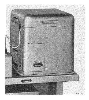
Reperforator TT-15/FG is an automatic teletypewriter receiving equipment which receives electrical impulses (according to the five-unit, start-stop teletypewriter code) and delivers messages so received in the form of perforated paper tape. It is used at army and higher headquarters.
