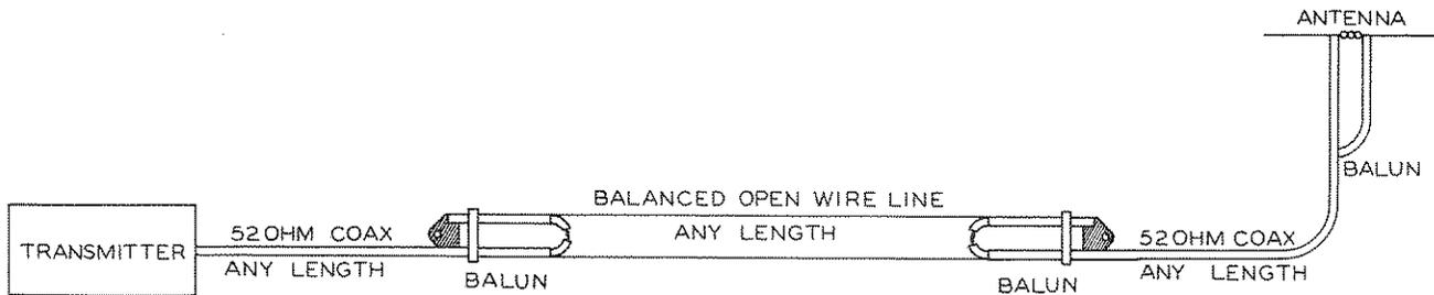
THIS SYSTEM PERMITS USE OF A BALANCED OPEN WIRE LINE TO REDUCE LOSSES ON LONG TRANSMISSION LINES. CONSTRUCTION DETAILS OF THE UNBALANCED TO BALANCED IMPEDANCE MATCHING TRANSFORMER (BALUN) USED BETWEEN THE OPEN WIRE LINE AND THE 52 OHM RG-8/U COAXIAL CABLE ARE SHOWN BELOW.
