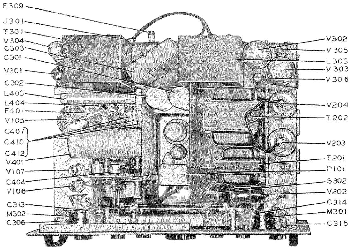
Figure 5-2 32V-3 Parts Arrangement - Top View
