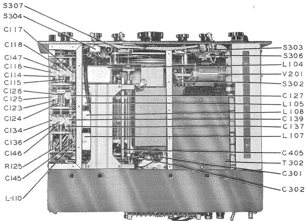
Figure 5-3 32V-3 Parts Arrangement - Bottom View
