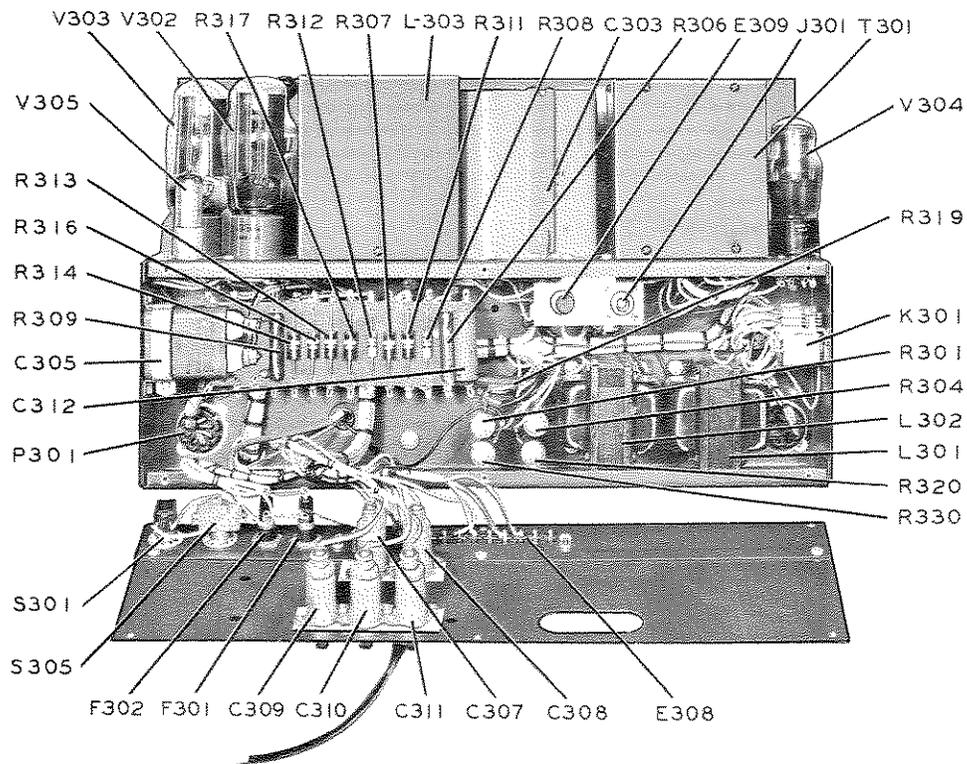
Figure 5-6 32V-3 Parts Arrangement - Rear Open
