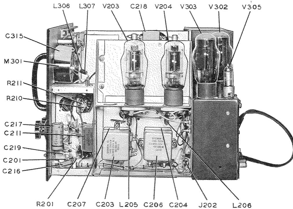
Figure 5-5 32V-3 Parts Arrangement - Right Side Open
