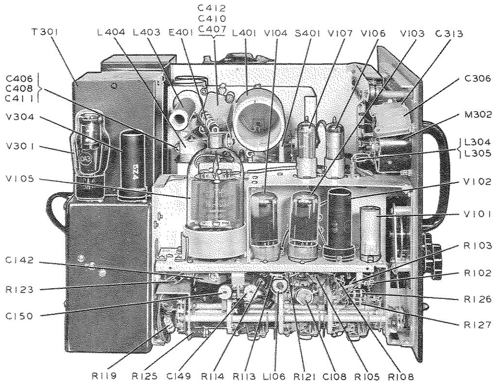
Figure 5-4 32V-3 Parts Arrangement - Left Side Open
