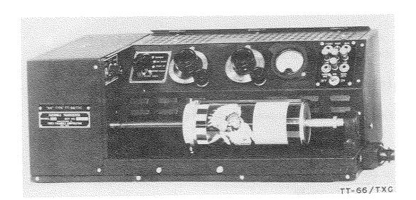
Facsimile Transceiver TT-66/TXC is a transportable, general purpose transmitting and receiving unit for communication by means of photographic, written, or drawn material.
