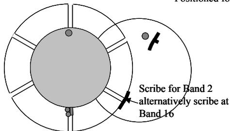
Radial Pin engages Stop pin for Band 16, 7 1/2 Turns past Band 1
