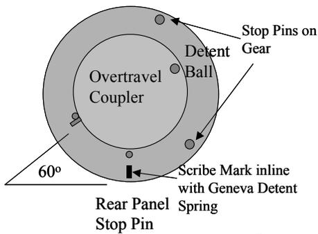
Stop Pins on gear under Geneva wheel
